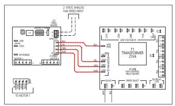
Figure 51 - Remove low voltage signal wires to motor(s)
