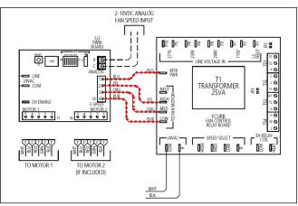
Figure 23 - Remove low voltage signal wires to motor(s)
