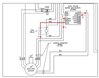
Figure 3 – Remove Motor Signal Wires
