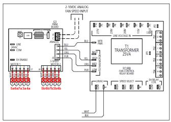
Figure 22 – Remove Motor Signal Wires
