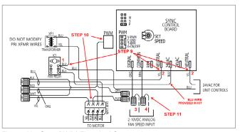
Figure 40 - Sync PWM Electrical Connections
