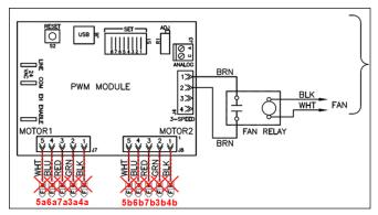
Figure 15 – Remove Motor Signal Wires
