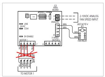
Figure 36 - Remove Motor Signal Wires
