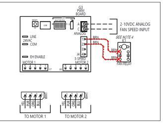
Figure 44 - Remove low voltage signal wires to motor(s)
