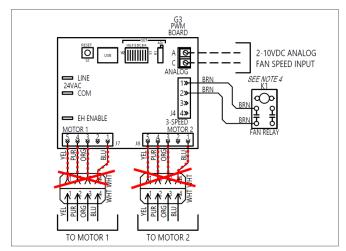
Figure 43 – Remove Motor Signal Wires
