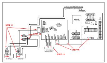
Figure 77 - Sync PWM Electrical Connections
