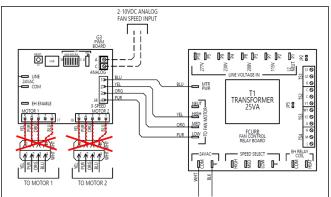
Figure 57 – Remove Motor Signal Wires
