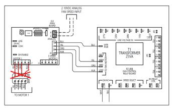
Figure 50 – Remove Motor Signal Wires
