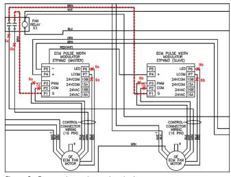
Figure 9 - Remove low voltage signal wires to motor
