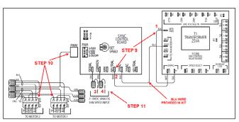
Figure 61 - Sync PWM Electrical Connections
