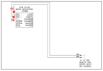
Figure 4 – Remove Motor Signal Wires
