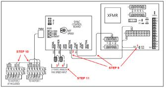
Figure 33 - Sync PWM Electrical Connections
