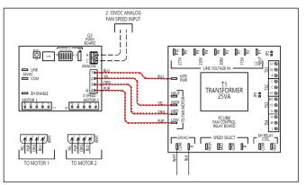
Figure 58 - Remove low voltage signal wires to motor(s)
