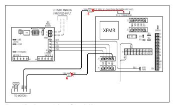
Figure 65 – Remove Motor Signal Wires
