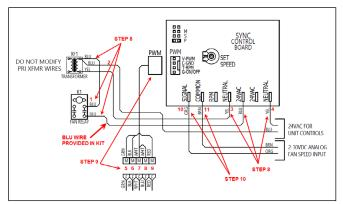
Figure 6 - Sync PWM Electrical Connections
