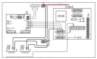
Figure 73 – Remove Motor Signal Wires
