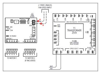
Figure 24 – Remove 2-10VDC motor control signal
