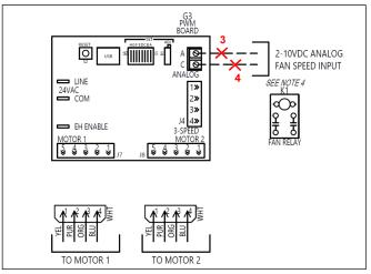
Figure 45 – Remove 2-10VDC motor control signal
