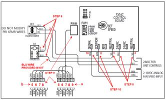
Figure 12 – Sync PWM Electrical Connections
