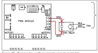
Figure 16 - Remove low voltage signal wires to motor(s)
