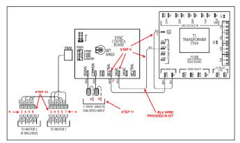
Figure 26 - Sync PWM Electrical Connections
