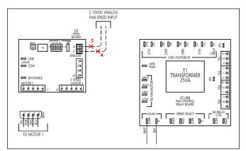
Figure 52 – Remove 2-10VDC motor control signal
