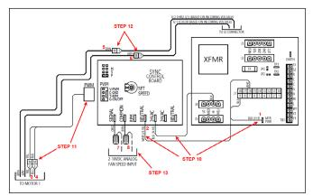
Figure 69 - Sync PWM Electrical Connections
