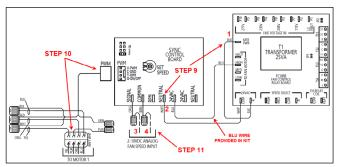
Figure 54 - Sync PWM Electrical Connections
