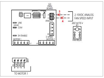
Figure 38 – Remove 2-10VDC motor control signal
