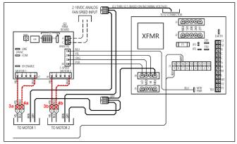
Figure 72 – Remove Motor Signal Wires
