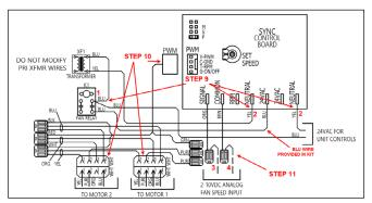
Figure 47 - Sync PWM Electrical Connections
