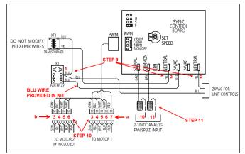
Figure 19 - Sync PWM Electrical Connections
