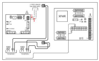
Figure 75 – Remove 2-10VDC motor control signal
