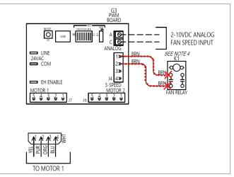
Figure 37 - Remove low voltage signal wires to motor(s)
