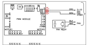
Figure 17 – Remove 2-10VDC motor control signal
