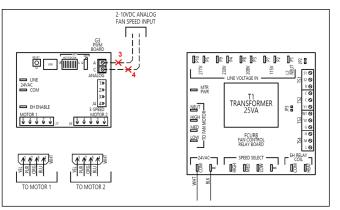
Figure 59 – Remove 2-10VDC motor control signal
