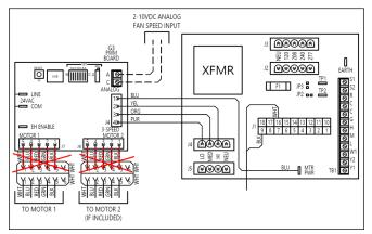
Figure 29 – Remove Motor Signal Wires
