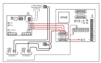
Figure 74 - Remove low voltage signal wires to motor(s)
