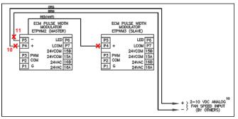
Figure 10 - Remove 2-10VDC motor control signal
