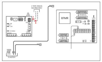
Figure 67 – Remove 2-10VDC motor control signal
