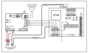
Figure 64 – Remove Motor Signal Wires
